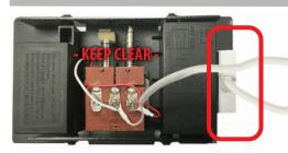
NOTE 1: Ensure that the power kit and wires DO NOT interfere with the mechanical parts of the chime.
