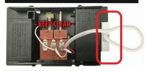
NOTE 1: Ensure that the power kit and wires DO NOT interfere with the mechanical parts of the chime.
