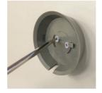
Feed the cable through the slot in the camera's base, align the locking tabs in the base with their matching slots on the underside of the camera; press firmly and rotate the camera in the clockwise direction to reattach the camera to the base.
